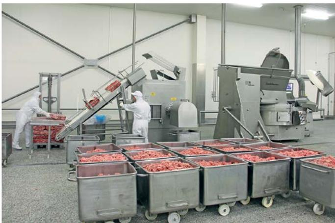
**At 800 kg of material per batch, the K 1004 AC-8 achieves a production capacity of 4.8 t or even more fine emulsion per hour.**
