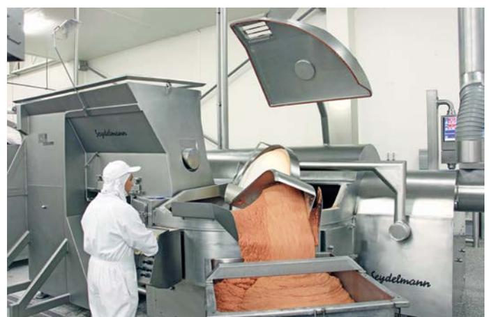
**The Belgian meat producer makes its complete assortment of products with the Seydelmann high-performance cutter.**
