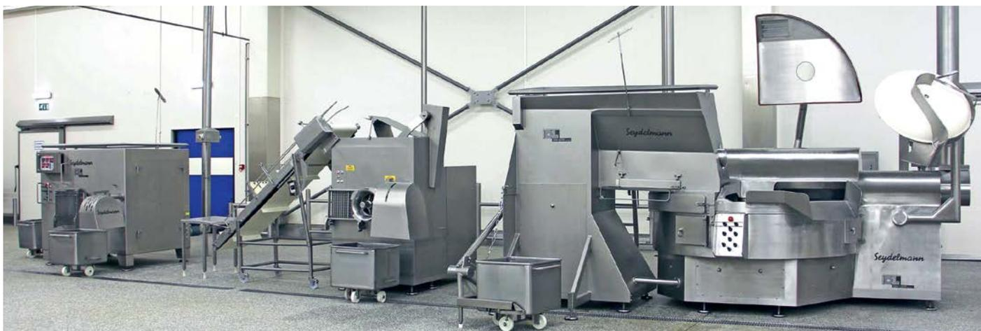
**Seydelmann machines: In addition to the 1,000-liter cutter, Vlevy uses four meat grinders and a 100-liter cutter made by the traditional Stuttgart company.**
